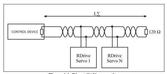
**Figure 4-1: Direct CAN connection**
