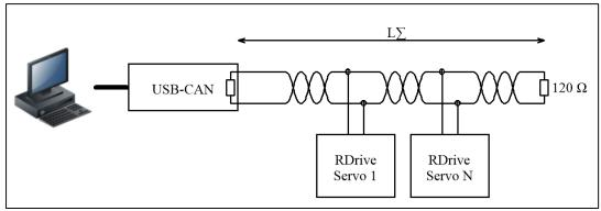
Figure 4-2: CAN-to-PC connection
